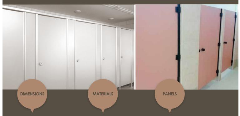
Cubicles' 2000mm overall height design includes a 150mm floor clearance. Its width and depth are tailored to meet your preferences and to adapt to individual site conditions. Standard design combines the use of solid compact laminate panel (phenolic core), natural anodized channel, and heavy duty stainless steel accessories. Other options are available.
